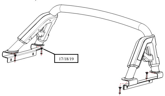
Step 4: Putting the roll bar on the Pick Up, adjusting the position, then marking and drilling 4 holes (Φ12) on the inside of carriage and install HEX NUT M12\*40.
