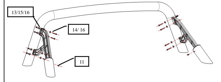
Step 2: Install the front and rear plastic cover with ST4.2\_30.
